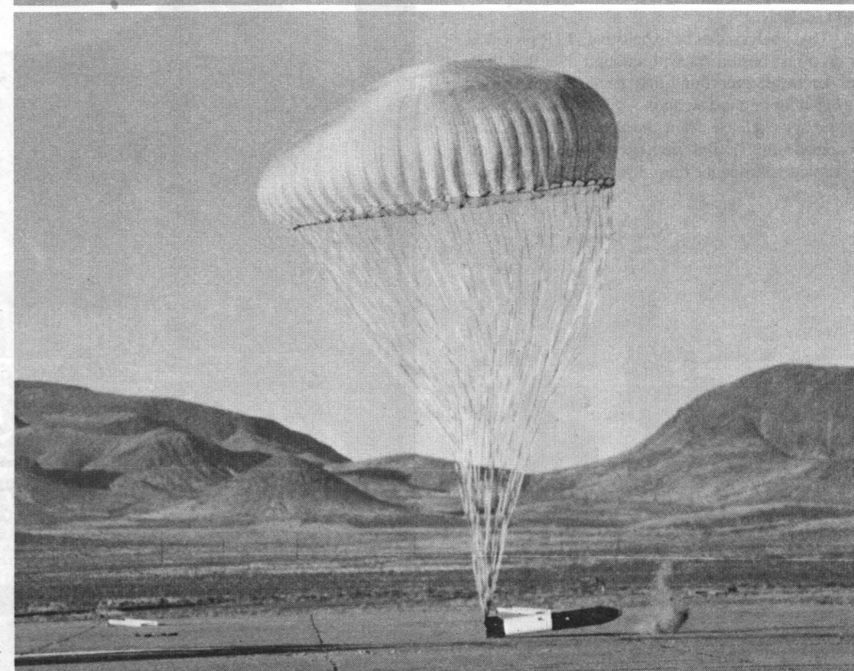
THIS DROP TEST series, which begins at upper left, shows a B83 parachute-retarded test assembly being dropped on a hard target at TTR from an FB-111.
